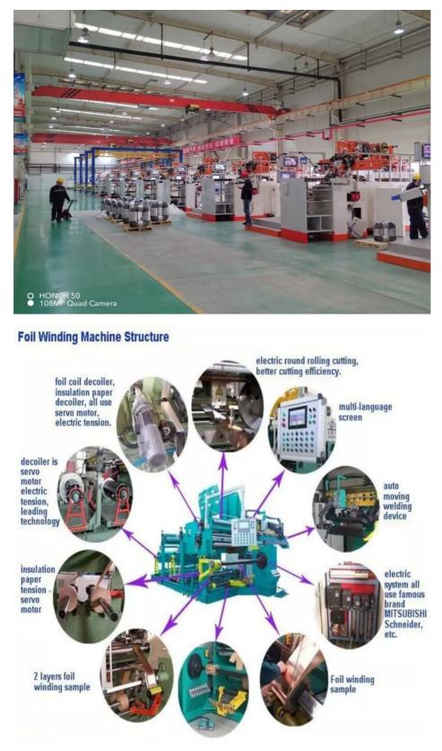
Single Layer Foil Winding Machine for 10 to 11ookv Insulators
