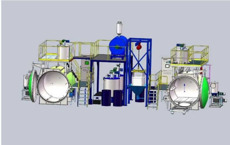
2. KCY-400-II vacuum pressure casting (the most commonly used in China)
