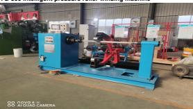
Features: This device is designed to solve the problem of excessive outer diameter of coils in domestic coil winding and on-site impact. The requirement level for employees is not high, which can lower the level of labor force. The pressure roller is driven by a servo motor, and the spindle speed is controlled by the system
