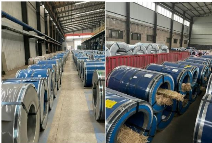
Baosteel CRGO B20r070 Laser Scribed Silicon Steel
