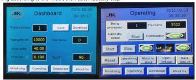
Motor is about: motor forward winding or backward winding. During winding, choose forward wind/backward winding according to product segment or non-segment technology.
