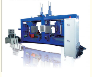
Double-station APG Clamping Machine
