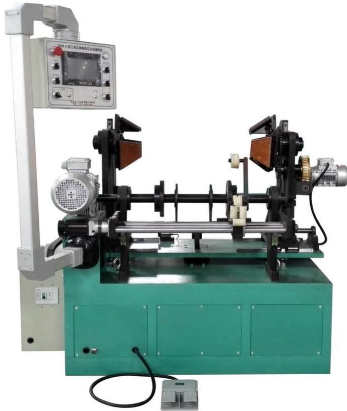
The High Voltage Automatic Winding Machine for 630KV Oil Transformer Coils with Intelligent High Pressure is a specialized piece of equipment designed for the precise and efficient winding of coils used in 630KV oil transformers. It incorporates advanced features and technologies to meet the specific requirements of high-voltage applications. Here are some key aspects of this machine:
