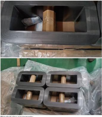
Manufacturing requirements: Tolerance: See demonstrated graphic; the specified requirements should be coincide with customers drawings; Material: we could choose Nippon steel, Baosteel, WISCO and other steel plants products to meet customers core loss requirements; in order to make sure we choose the right material, we would like our customers to provide us with detailed drawings including necessary technical parameters. Usually, we use 0.18mm, 0.20mm, 0.23mm, 0.27mm, 0.30mm material.
